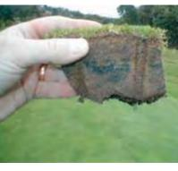
Very limited oxygen transfer from hollow core
